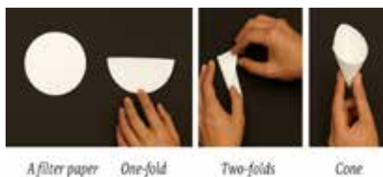
Figure : Folding a filter paper to form a cone
