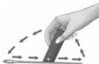
(a) Making an iron needle a magnet
