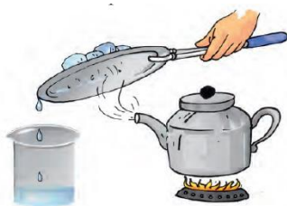
Fig. 3.13 Evaporation and condensation
